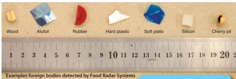
The Food Radar system is presently operational on four continents serving several major global producers. We have a fully equipped pilot plant in Gothenburg, Sweden where our customers can test the systems capability to detect foreign bodies in their own products.
