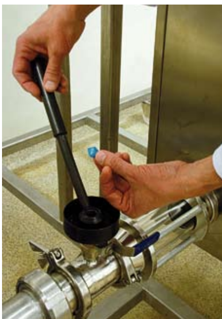
Picture 8: "Customers can test their own products by inserting their own foreign bodies in the pilot plant"
