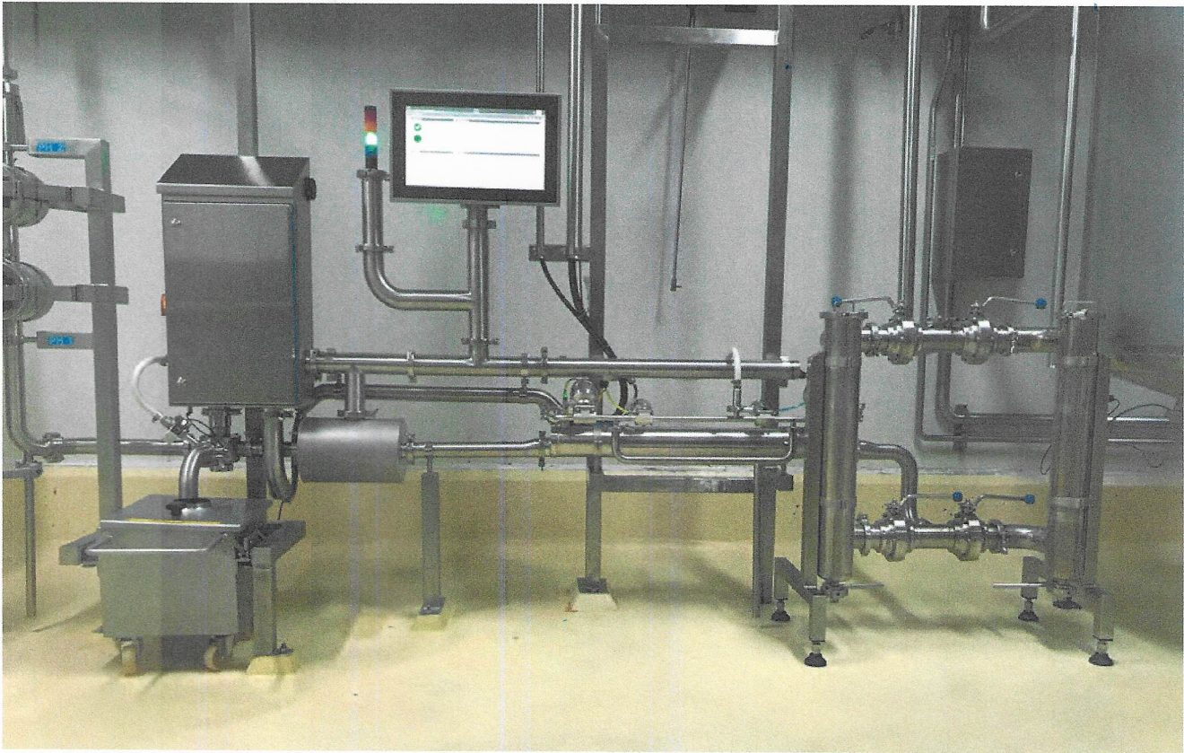
The 'Food Radar' quickly detects and removes previously undetectable foreign bodies from food production lines
