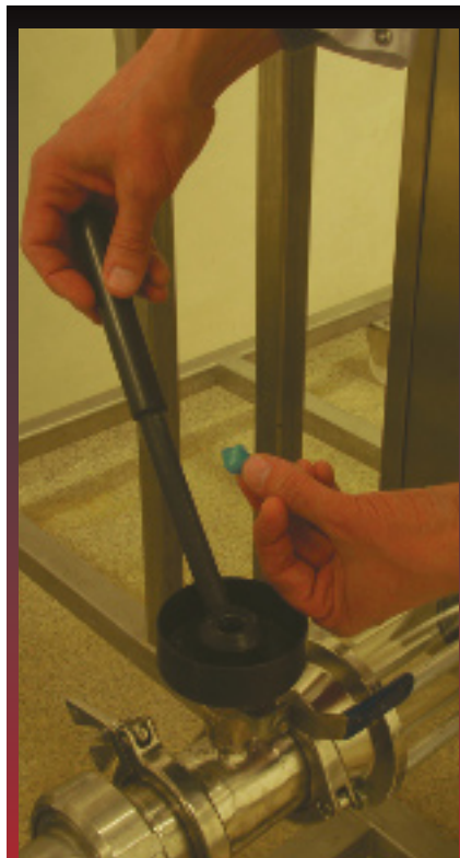
Customers can test their own products by inserting their own foreign bodies in the pilot plant
