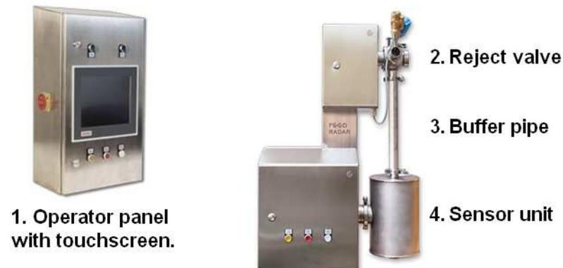
All system components are hygienically contained in stainless steel cabinets, which are IP65 classified or higher. The sensor does not have any moving parts, and the rejection unit is a three-way valve, which has been certified by the European Hygienic Engineering & Design Group. The entire system takes up about one metre of pipe length and is, therefore, very convenient and easy to install leaving a minimum footprint.
